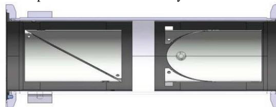
Figure 2: Cross section view of the ELENA Pick-up.
