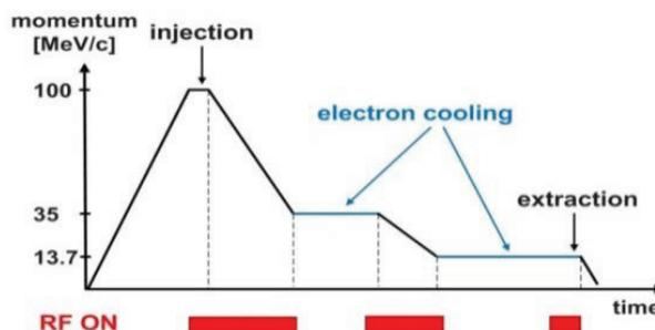
Figure 1: Schematic view of the ELENA cycle.
