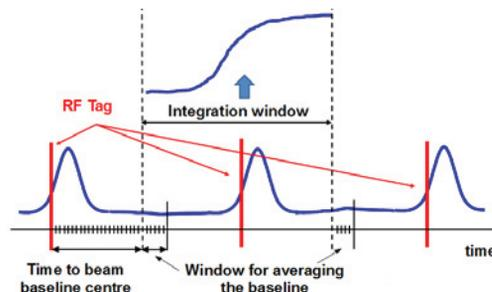
Figure 6: Integration window for bunched intensity measurements.
