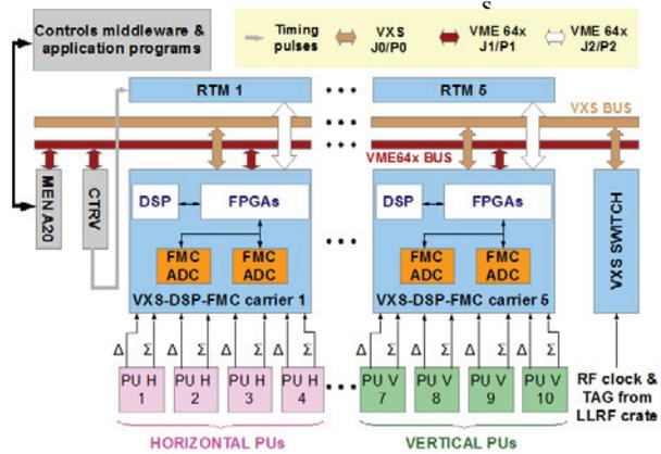
Figure 4: Digital acquisition system block diagram. ADC: Analogue-to-Digital FMC board. RTM: Rear Transition Module. CTRV: Timing Receiver Module. Men A20: master VME board. PU H: Horizontal transverse Pick-Up. PU V: Vertical transverse Pick-Up.
