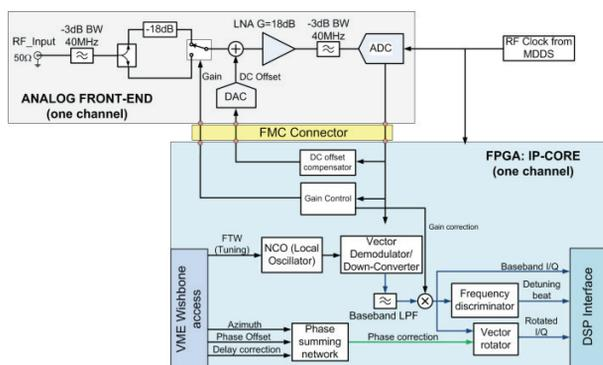
Figure 5: FMC-ADC board hardware and DDC firmware.
