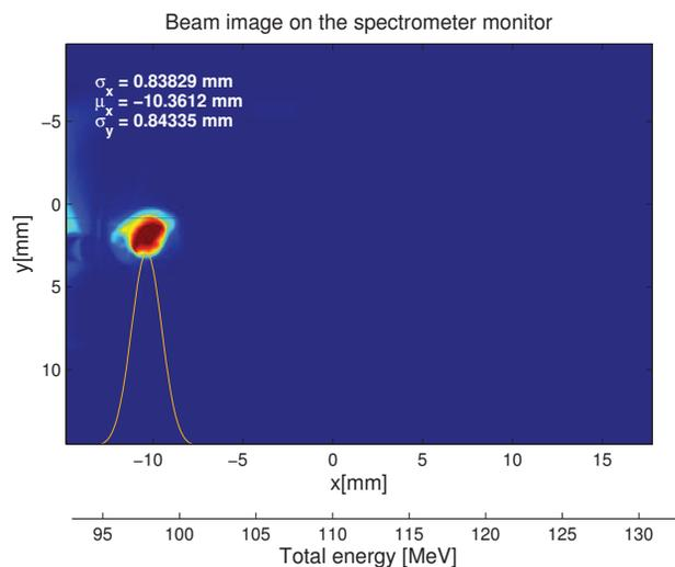
Figure 3: The electron beam image captured at the spectrometer camera. The x-position of the beam is used to estimate the beam energy.
