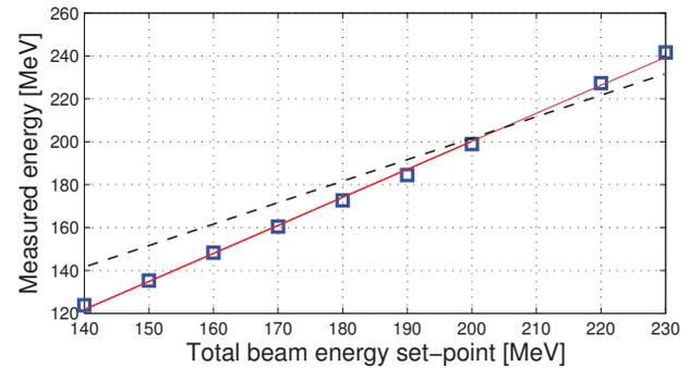
Figure 2: The total measured beam energy versus the reference (setpoint) energy. The dashed-line, which simply plots the equation  $y = x$ , represents the ideal open-loop response.
