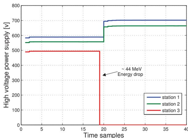
Figure 5: The high voltage value of the three klystrons at the SwissFEL injector test facility.
