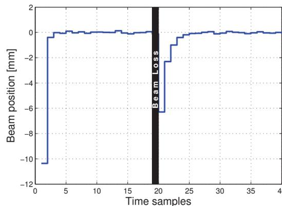
Figure 4: The beam position measured on the spectrometer monitor. The zero position corresponds to the desired energy which, in this case, is 110 MeV.
