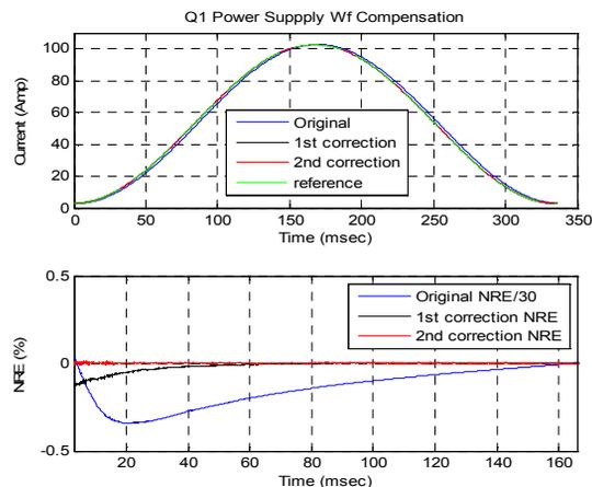
Figure 7: The upper plot is output waveform and the lower plot is NRE during three iterations of correction for Q1. It only required ones correction to achieve 0.2 % NRE.
