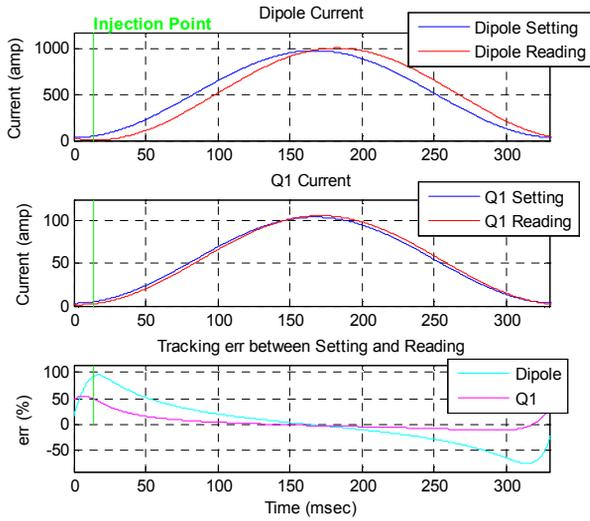
Figure 3: Ramping waveform of Dipole and Q1. Different phase delay will cause different tracking error between setting and reading.
