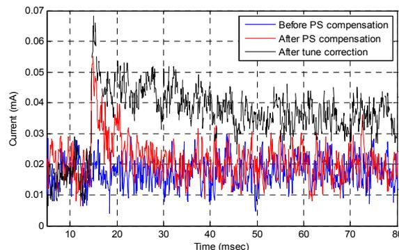
Figure 8: Booster beam current comparison before and after power supply waveform compensation and tune correction at single bunch mode.
