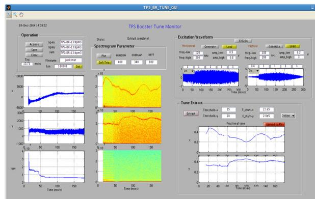
Figure 9: Tune monitor during Booster ramping before tune compensation. Vertical tune variation was as large as 0.25.
