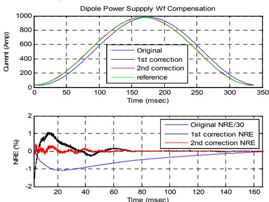
Figure 6: The upper plot is output waveform gradually closed to reference and the lower plot is NRE gradually decreased during three iterations of correction for Dipole.
