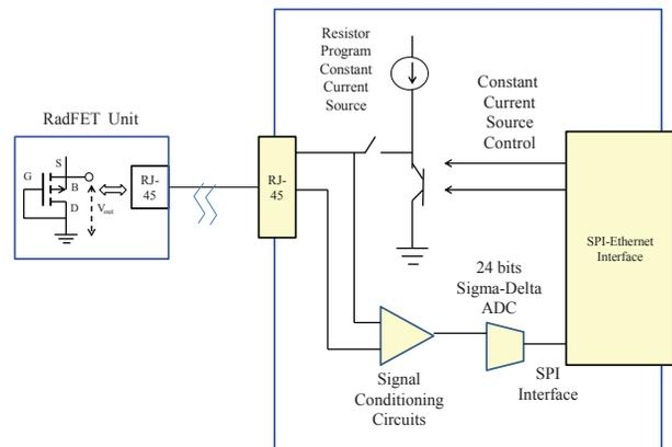
Figure 1: Simple schematic diagram of an individual RadFET reading hardware.
