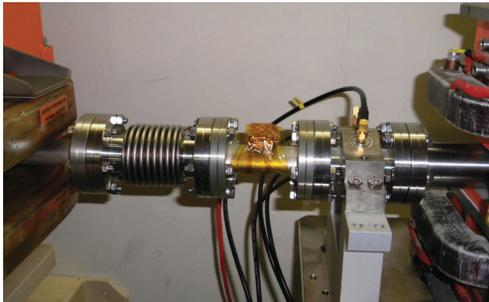
Figure 4: Typical installation for RadFET sensors.
