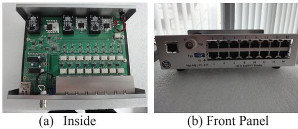
Figure 3: Photo of the 16 channel RadFET reader.
