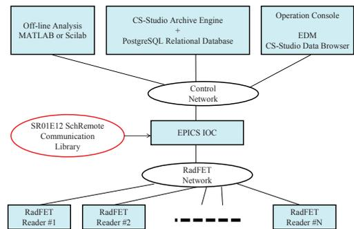
Figure 5: Software support for RadFET reader.
