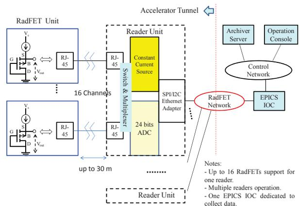
Figure 2: Block diagram of the RadFET readers system.
