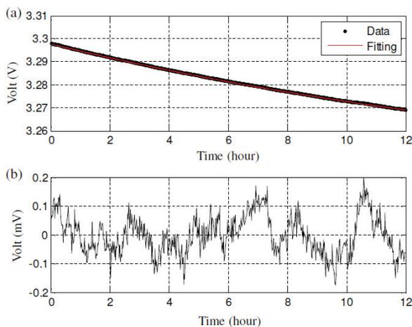
Figure 10: (a) Threshold voltage and its fitting curve during non-radiative period. (b) Voltage fluctuation within 12 hours.
