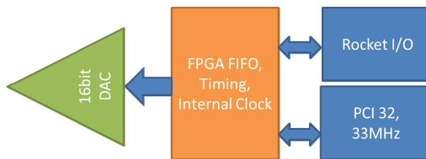
Figure 4: Functional block diagram of the corrector power supply control interface module. The fast setting from feedback engines will sum with slow setting from ILC.
