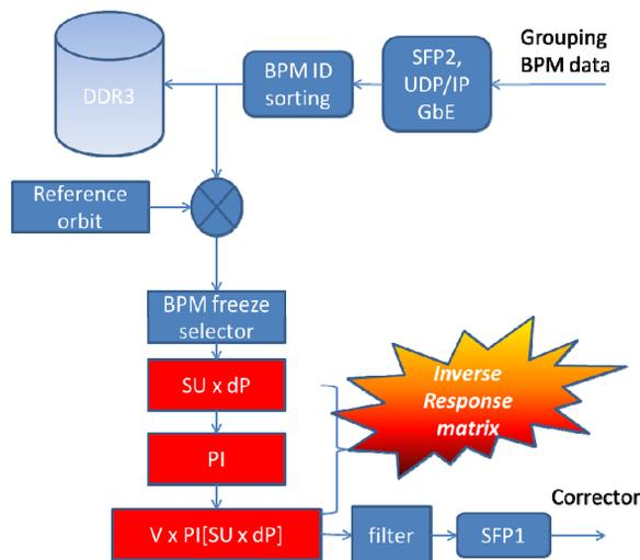
Figure 6: Control algorithm block diagram.
