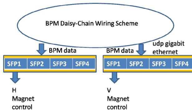
Figure 2: Feedback system is integrated by daisy-chain wiring bus of bpm with GDX module.
