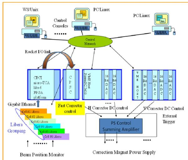
Figure 1: The overview system block diagram.
