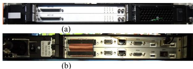
Figure 5:(a) CPSCI AO32 frontend. (b)CPSCI AO32 backend. 32 channels AO is extend to 64 channels AO by RTM-AO16 bus.
