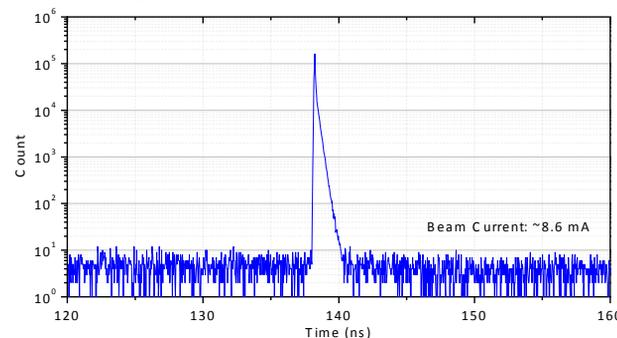
Figure 11: Preliminary single bunch purity measurement by time-correlated single-photon counting technique.
