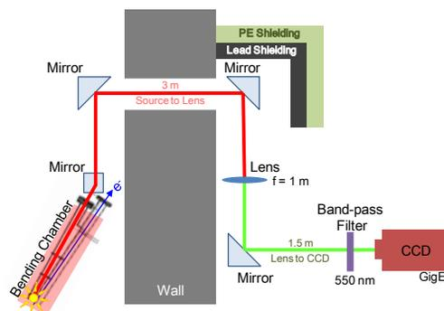
Figure 1: A side-view scheme of the synchrotron radiation monitor for the booster ring.
