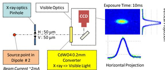
Figure 6: The pinhole camera parameters and measurement result under the single bunch mode. The storage beam current  $\sim 2$  mA, the pinhole is set to  $50$   $\mu\text{m} \times 50$   $\mu\text{m}$ ; CCD exposure time is 10 ms.
