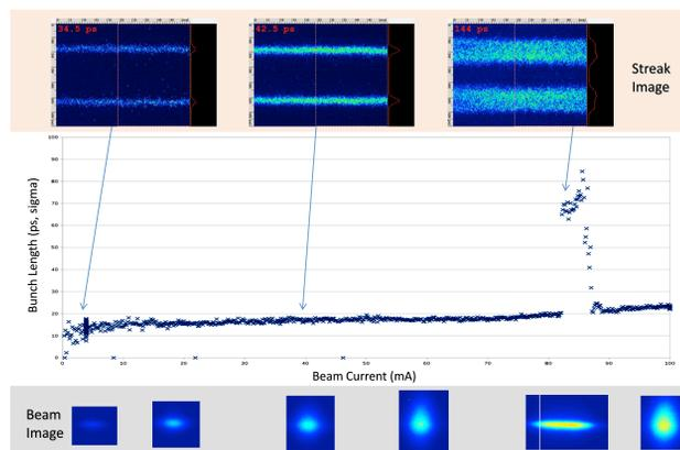
Figure 10: Longitudinal instability observation under multi-bunch via streak camera and X-ray pinhole camera.
