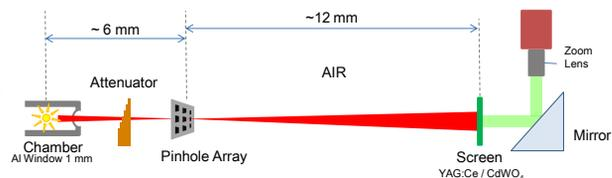
Figure 2: A side-view scheme of the X-ray pinhole camera for the storage ring.
