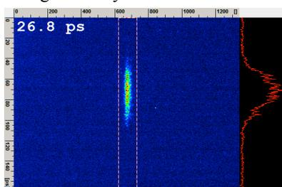
Figure 8: Typical streak image of bunch length measurement at TPS storage ring under single bunch mode, the bunch length ~26.8 ps (FWHM), storage beam current ~2 mA, vertical scale = 150 ps.
