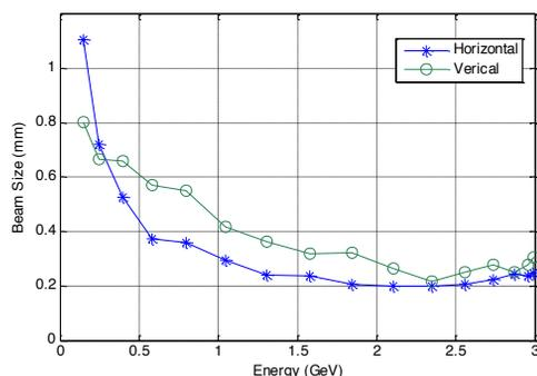
Figure 5: Measured variation of beam size with energy ramping of booster synchrotron.
