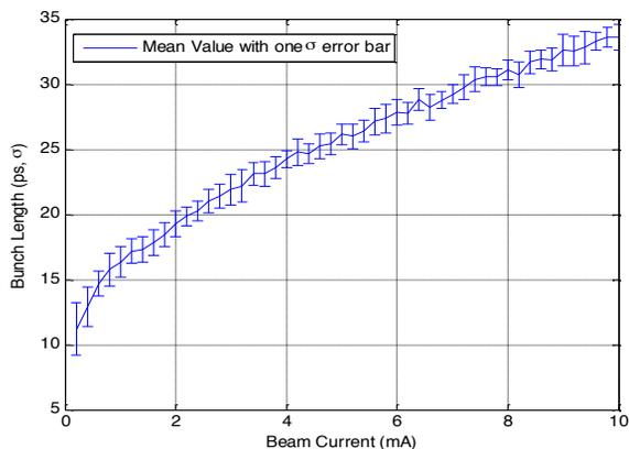
Figure 9: The relative relationship between the beam current and bunch length under the single bunch mode.
