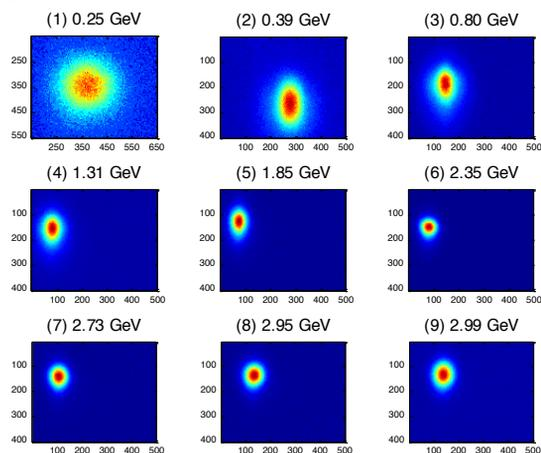
Figure 4: TPS booster synchrotron radiation profiles at varied energy ramping point, 1 pixel is around 9  $\mu\text{m}$ .
