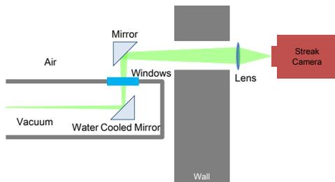
Figure 3: A top-view scheme of the visible light synchrotron radiation monitor for the storage ring.
