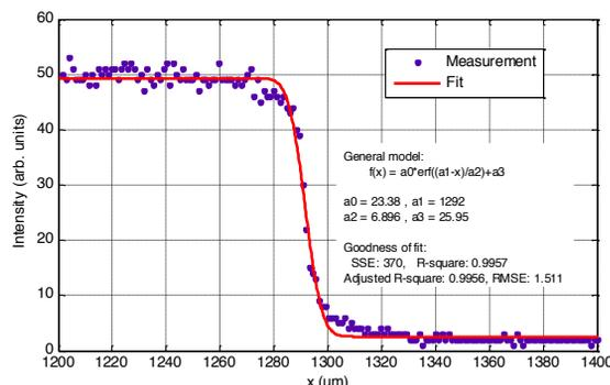
Figure 7: Resolution measurement of the X-ray pinhole camera, the resolution  $\sigma_{\text{screen}} \approx 5$   $\mu\text{m}$ .
