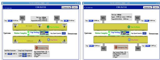
Figure 4: EDM based TLS U50 and U90 control GUI.
