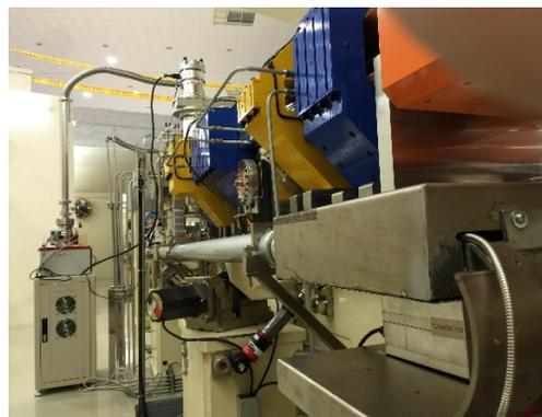
Figure 2: Laser portion and isolation tube of Laser-PSD system are assembled on the side of girder in lab. Then magnet girders are transported back and placed on pedestals in TPS tunnel.
