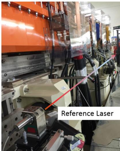
Figure 9: The reference PSD will be installed on girder for adjusting the reference laser to parallel to the datum plane of front girder.
