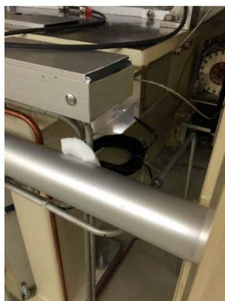
Figure 5: When the sponge obstructs the water pipe vibration, the PSD stability is improved immediately.
