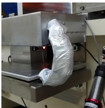
Figure 4: The Laser fiber is fastened by thermal insulation material.
