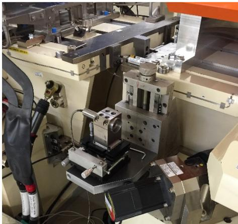
Figure 8: The reference laser is set on pedestal for recalibration.
