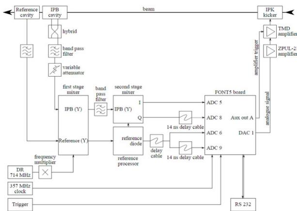
Figure 4: Schematic of configuration of IP feedback system.
