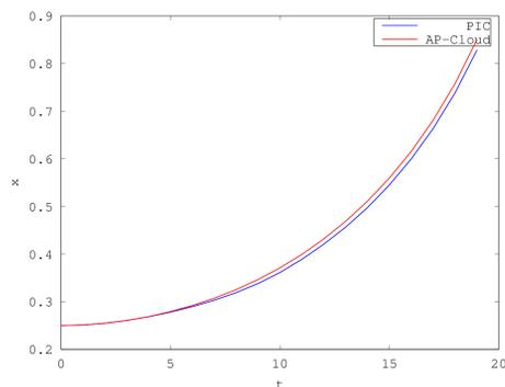
Figure 5: Motion of a single test particle obtained with PIC and AP-Cloud methods demonstrating the absence of artifacts in the AP-Cloud method.
