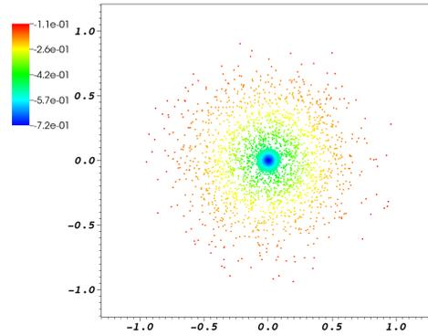
Figure 1: Typical distribution macroparticles in transverse cross section of accelerator beam with halo. Color represents numerical solution values for the potential.
