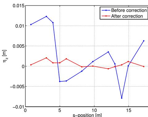
Figure 5: Vertical dispersion of the initial (with simulated quadrupoles tilt) and corrected lattice.
