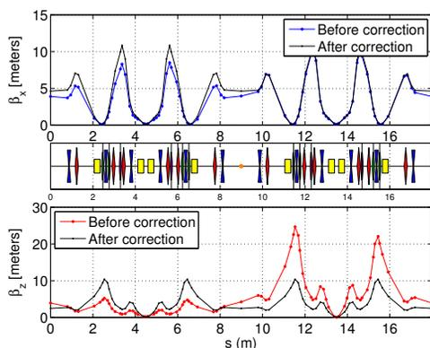
Figure 4: Beta functions of the initial (with simulated errors) and calibrated to the nominal ThomX SR lattice models.
