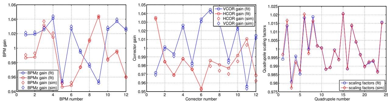
Figure 3: LOCO fitting results: comparison of the BPM gains, correctors gains (i.e. corrector kicks as a fraction of the intended kicks) and the quadrupole strength scaling factors with the corresponding values applied as the errors to the model.
