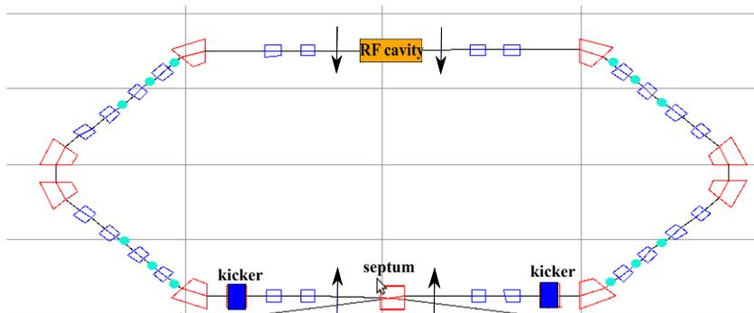
Figure 3: Layout of the ThomX ring with 4 octupoles to increase the DA and MA. The red trapezoids are dipoles; the blue rectangles are quadrupoles, the cyan dots are sextupoles; the down arrows are the defocusing octupoles, and the up arrows are the focusing octupoles.
