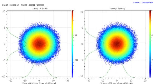
Figure 3: Beam output phase-space distributions in  $(x, x')$  and  $(y, y')$ ; T1-T3 beam lines of config1.
