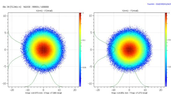
Figure 6: Beam output phase-space distributions in  $(x, x')$  and  $(y, y')$ ; T3 beam line of config2.
