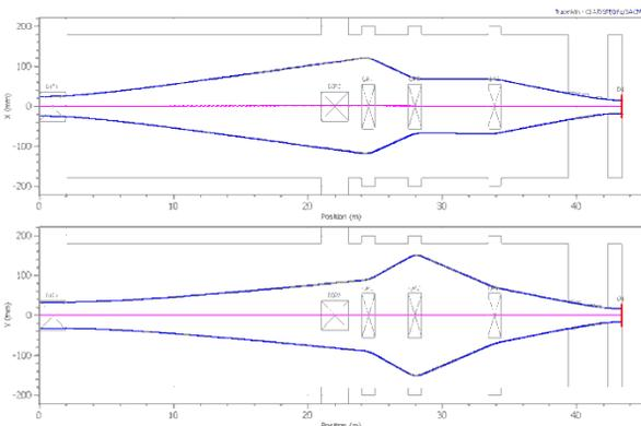
Figure 2: Beam envelopes ( $4\sigma$ ) – T1 axis (config1).
