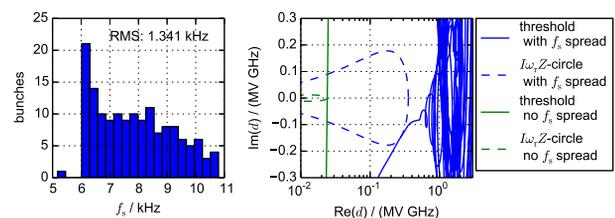
Figure 6: Left: Distribution of the synchrotron frequency of the long bunches. Right: Complex plane of the dispersion function at the instability threshold (solid lines) and  $I\omega_r Z$ -circles (dashed lines) indicating the maximum current.
