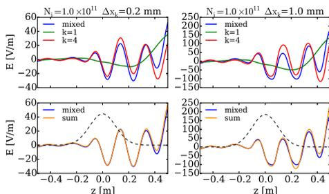
Figure 2: Electron cloud wakefields generated by the perturbed bunches with modes  $k = 4$  and  $k = 5$ . Upper plots show the simulation results for each mode separately and for the mixed modes with the same amplitude. Lower plots compare the sum of the single mode wakefields with the simulations for the mixed mode.
