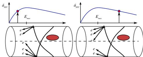
Figure 6: Secondary emission process for different bunch populations/SEY maximum position.
