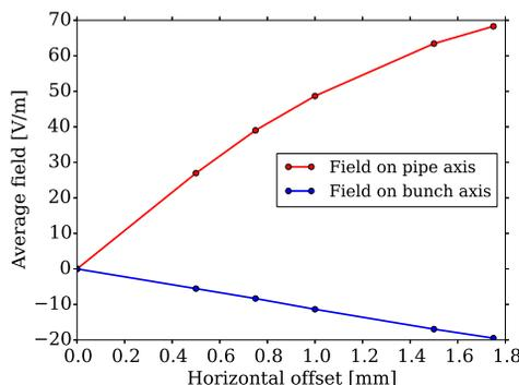
Figure 3: Electron cloud transverse fields in cylindrical geometry averaged over bunch longitudinal profile on bunch axis (blue) and on pipe axis (red). The pipe is cylindrical and  $N_i = 10^{11}$ .
