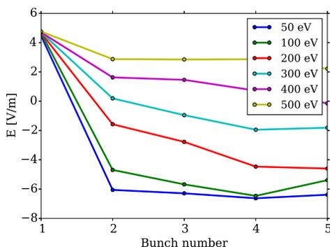
Figure 7: Electron cloud transverse fields on bunch axis averaged over bunch longitudinal profiles for several positions of SEY maximum. The LHC dipole geometry is assumed. The cloud is initially uniform with density  $10^9 m^{-1}$ .
