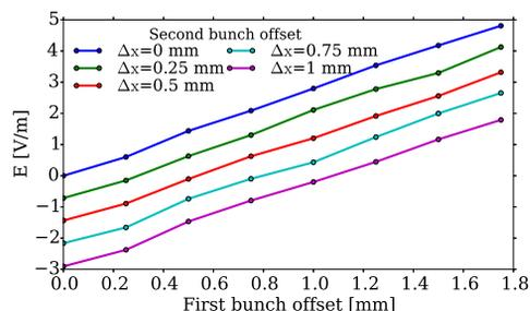
Figure 8: Electron cloud transverse fields averaged over the second bunch profile, excited by  $k = 0$  mode of the first and second bunches in bunch train. Initial cloud distribution is uniform.
