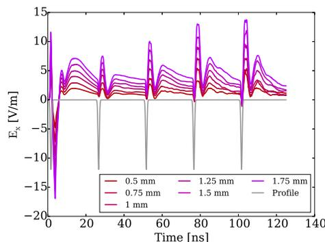
Figure 4: Electron cloud transverse fields on pipe axis excited by  $k = 0$  mode of the first bunch in bunch train, in presence of dipole magnetic field. Initial cloud distribution is uniform. The offset is horizontal.
