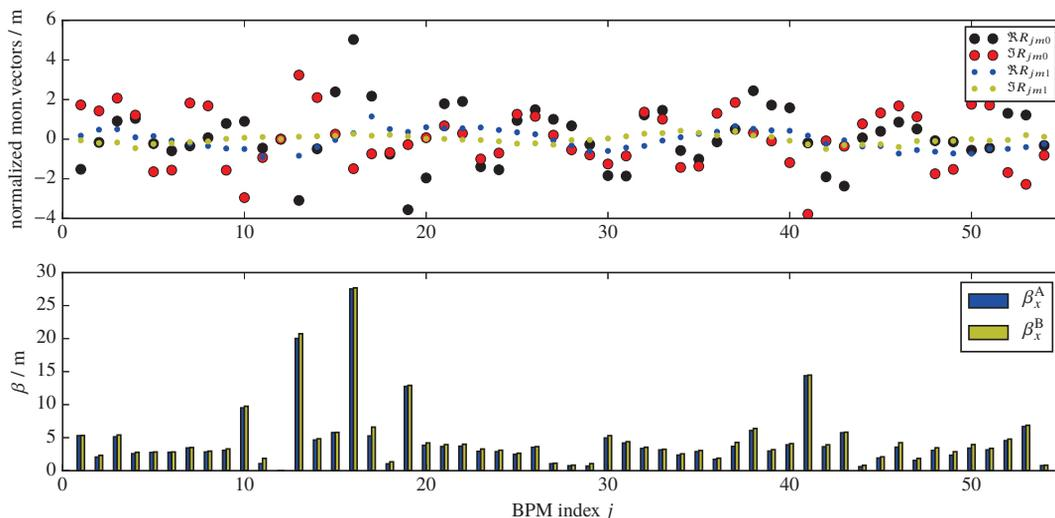
Figure 2: Preliminary results for invariant-normalized optical parameters in mode  $m = 0$ . The upper plot shows normalized monitor vector components, the lower plot shows two different estimates for the decoupled  $\beta_x$  function. ( $j = 12$  defunct.)
