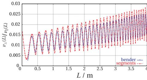
Figure 3: Ratio of transversal and parallel velocities of a design particle in the adiabatic injection channel.
