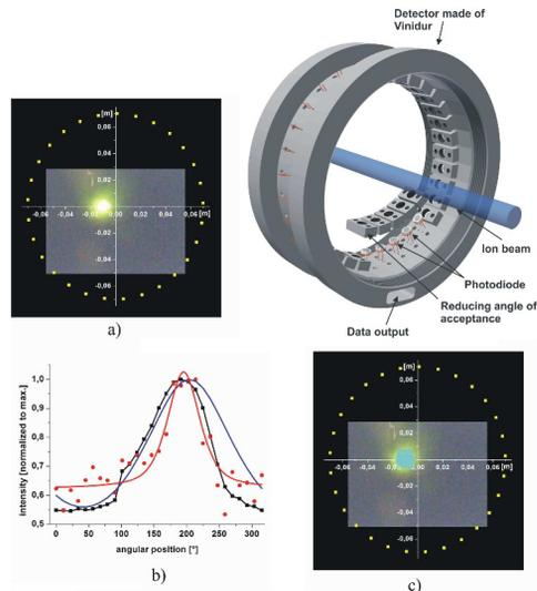
Figure 7: a) Beam on the scintillation screen within the coordinates of the vacuum vessel and the photodiode-detector in yellow. b) Approximation of experimental results (red), scintillation screen data (black) and simulated data (blue). c) The simulated luminescence distribution (cyan) is mapped on the scintillation screen picture for comparison and proving the detection of position and diameter of the beam.
