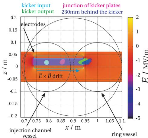
Figure 5: Kicker area with beam monitor profiles of the shifted injected beam.
