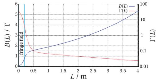
Figure 2: Rise of the magnetic flux and the adiabatic condition, on axis along the injection channel.
