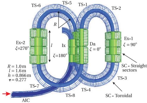
Figure 1: Figure-8 Storage Ring with the proposed adiabatic injection channel (AIC).
