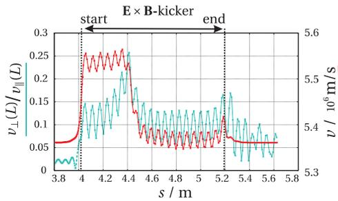
Figure 4: Ratio of transversal and parallel velocities and the total velocity of a design particle in the  $\mathbf{E} \times \mathbf{B}$ -kicker.
