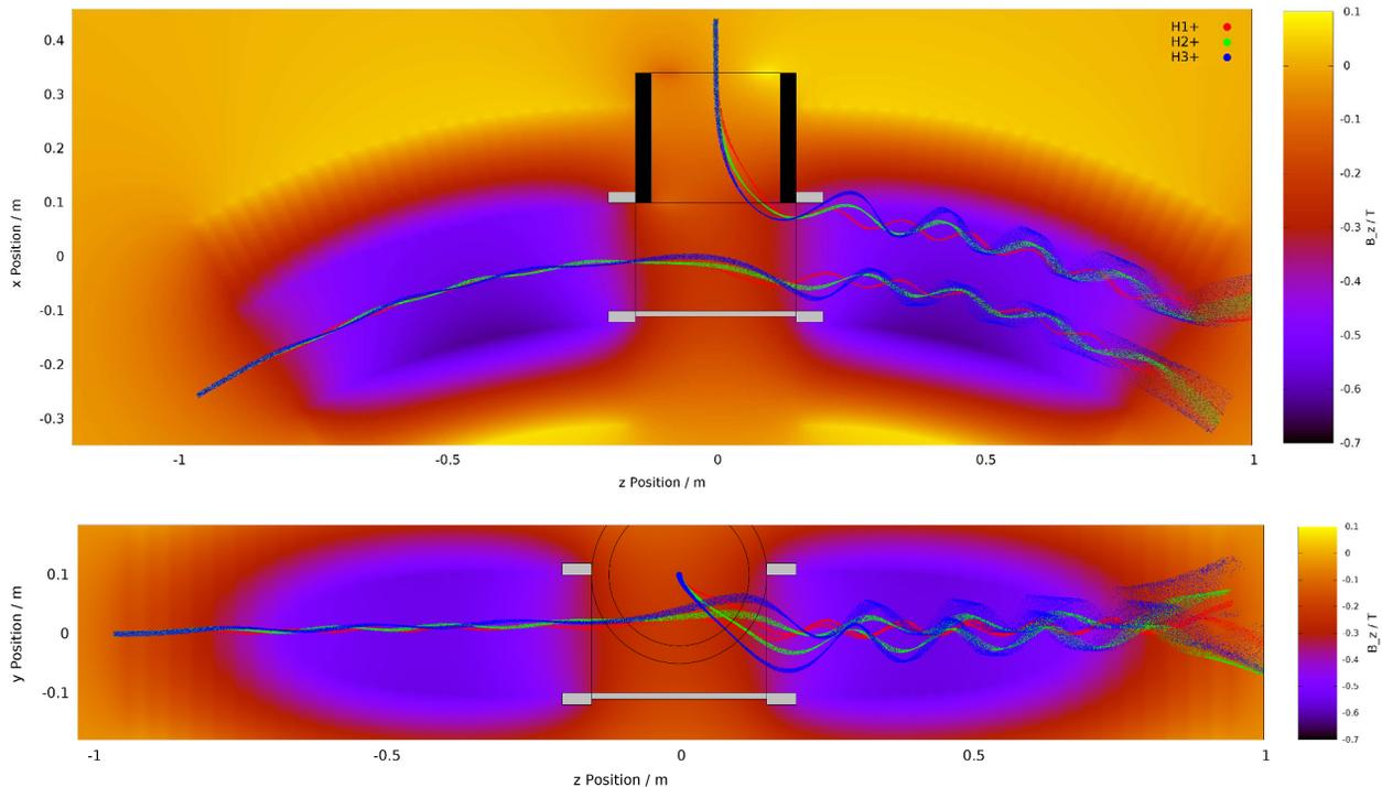
Figure 8: Particle simulations using the multi-particle code *bender*: Simulation of the injection experiment using two 7.8 keV hydrogen ion beams, two toroidal magnets with 0.6 T and a solenoidal injection coil with 0.2 T.
