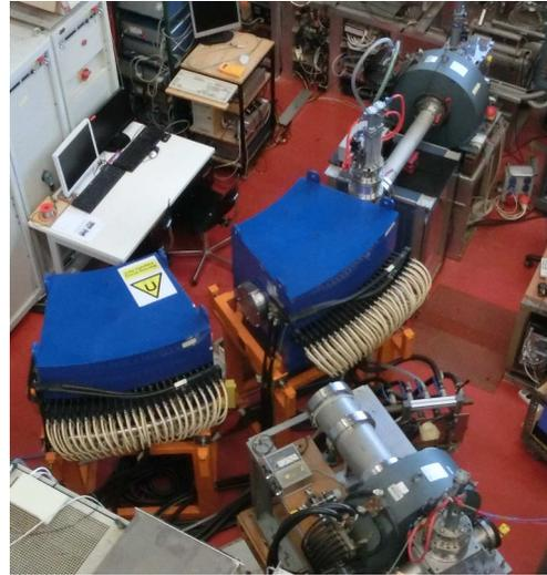
Figure 6: Top view picture of the scaled down experiment at Frankfurt University with two ion sources.
