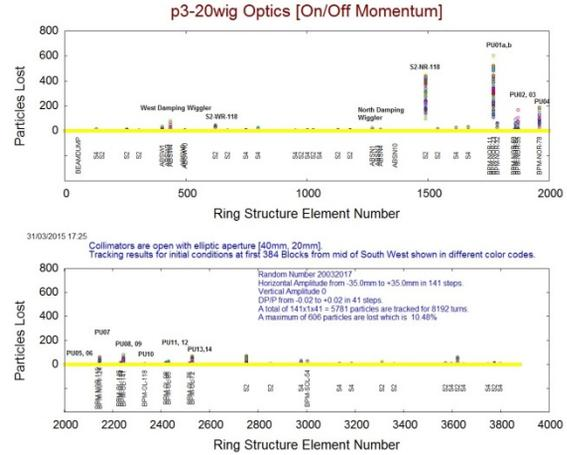
Figure 5: Tracking results for off momentum particles.
