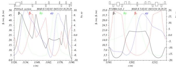
Figure 4: The computed values of  $a_y$  and  $b_y$  are plotted for the sections for sector (a) PU01 and (b) PU02. The  $a_y$  value is high at the upstream of PU01 and PU02; as well as downstream of PU01 and PU02.
