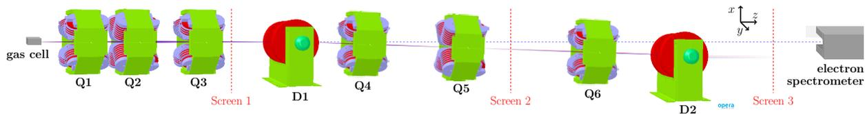
Figure 1: Sketch of the setup with six quadrupoles and two dipoles. The beam profile was measured with scintillating screen 1 to 3, the energy distribution with the electron spectrometer.
