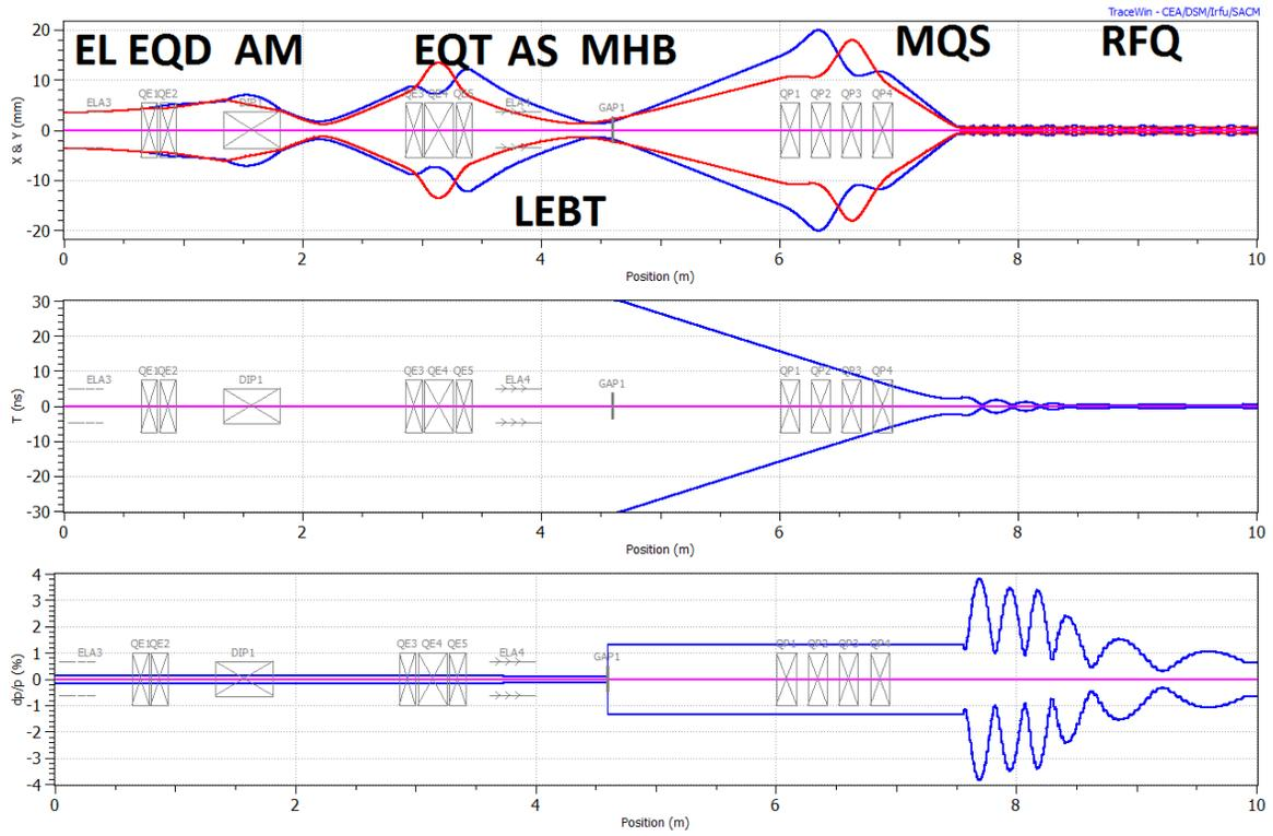
Figure 1: Beam Optics of LEBT+ RFQ section.
