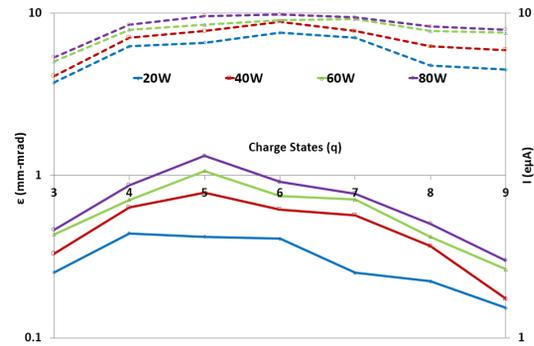
Figure 2: Argon ion spectrum at different RF powers.
