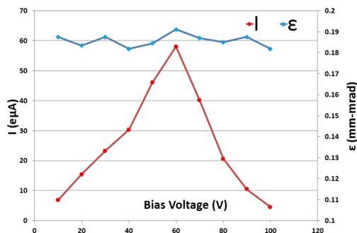
Figure 4: Emittance versus bias voltage of inserting electrode into ECR plasma.
