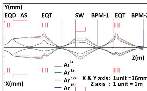
Figure 1: Beam optics of LEIBF in 90° line using TRANSPORT code for charge states of Ar ion beam at the energy of q\*210 keV.
