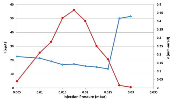
Figure 3: Emittance versus injection pressure of the Ar gas.
