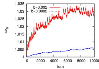
Figure 5: Emittance growth of the model with Eqs.(17) and (18).
