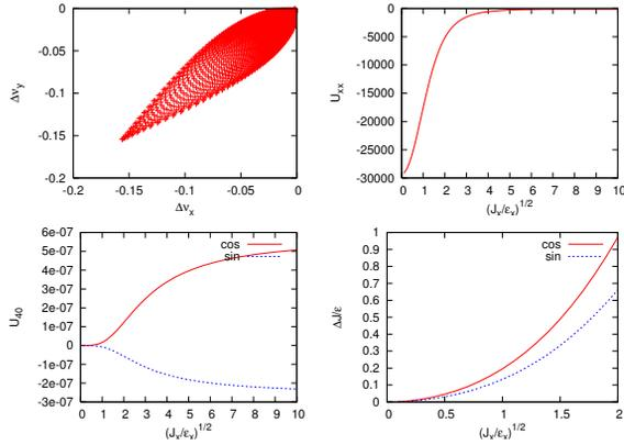
Figure 1: Tune spread ( $\Delta\nu_{x,y}(J_x, J_y)$ ), slope ( $\partial^2 U_0 / \partial x^2$ ), 4-th order resonance strength ( $U_{4,0}$ ) and its width due to space charge force as function of  $J_R$ .
