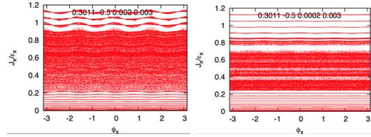
Figure 4: Phase space trajectory for the model map taking into account of effective synchrotron motion, Eqs.(17) and (18). Left and right plots correspond to parameters (1) and (2), respectively.
