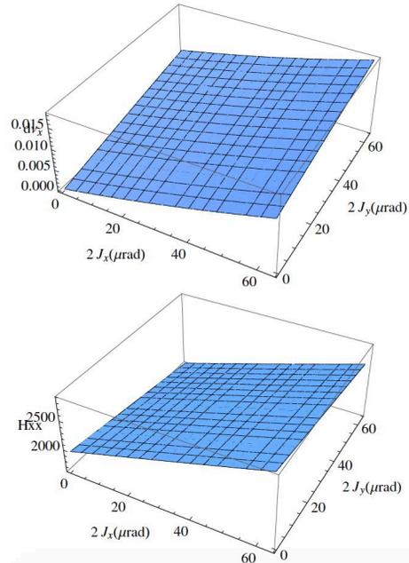
Figure 2: Tune spread,  $\partial^2 U_{00} / \partial x^2$  induced by lattice nonlinearity.
