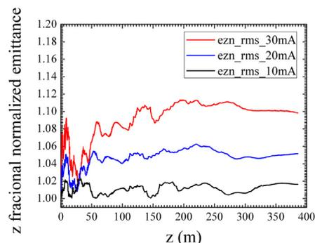
Figure 2: Longitudinal normalized rms emittance growths of the main linac basic design with different average beam current on basis of Injector I scheme.
