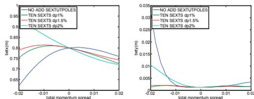
Figure 6:  $\beta$  function bandwidth for optimization in CEPC FFS.
