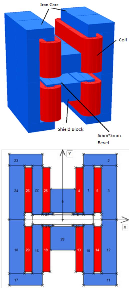
Figure 1: The 3D model of the new type of magnet (top) and the central plane of the magnet (bottom).
