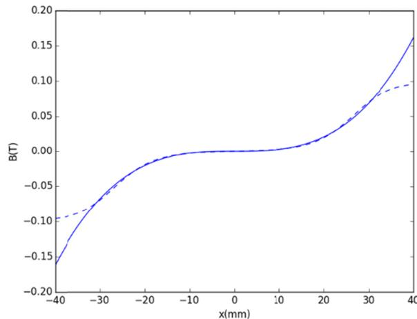
Figure 2: The magnetic field profiles with the minimum (top) and maximum (bottom) distance (dash line) between the two C-type dipoles compared with octupole (solid line).
