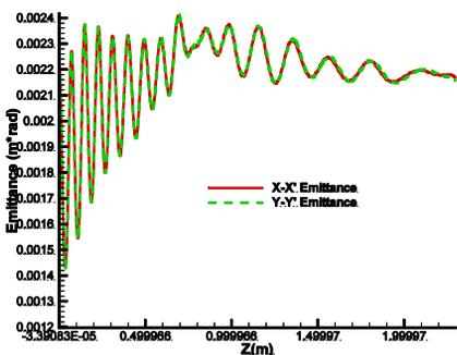
Figure 5: Emittance variation along the DTL.
