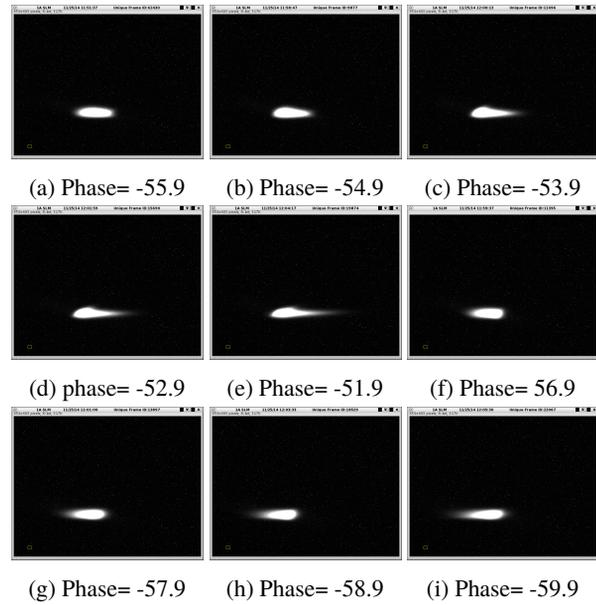
Figure 1: The size of the spot on SLM changes as the NL gang phase changes.
