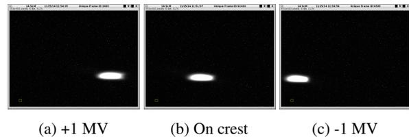
Figure 2: Changing the gradient by  $\pm 1$  MV to calculate the dispersion.
