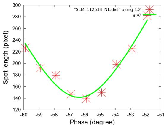
Figure 3: Hyperbola fitting for head to tail calculation.
