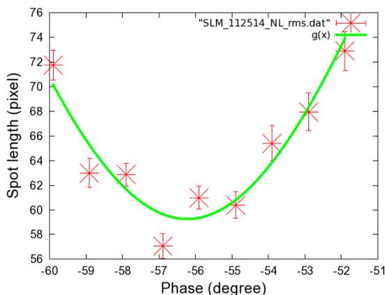
Figure 4: Hyperbola fitting for RMS calculation.
