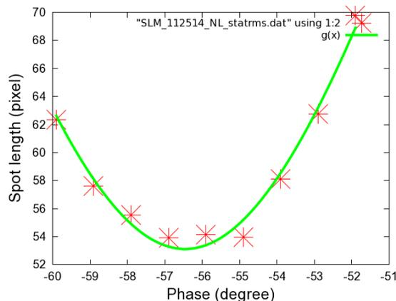
Figure 5: Hyperbola fitting for stat. RMS calculation.
