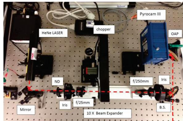
Figure 3: Optics setup to test and align the CDR AD imaging system for ALICE.
