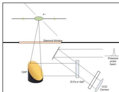
Figure 5: Proposed EO far field CDR AD electro-optic imaging system.
