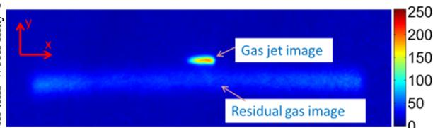
Figure 2: Beam profile from the supersonic gas-jet monitor.
