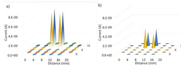
Figure 4: A 5 MeV  $Fe^{++}$  beam through a slit of 8mm x 8mm at the highest current measurement for a (a) raster scanned (392 nA at FC2); and (b) a defocused (184 nA at FC2).
