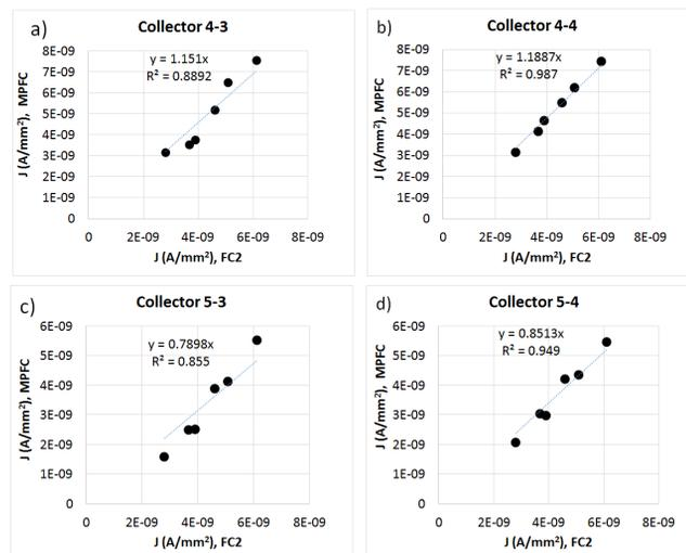
Figure 5: Measurements of current density using FC2 after the slit apertures and the MPFC device for the raster scanned ion beam. The MPFC device collectors (in a given area) responded in a linear pattern to variation in the total beam current, and correlate well to the current density of a traditional suppressed Faraday cup.
