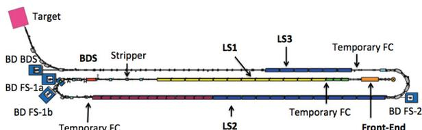
Figure 1: Schematic layout for FRIB driver linac.
