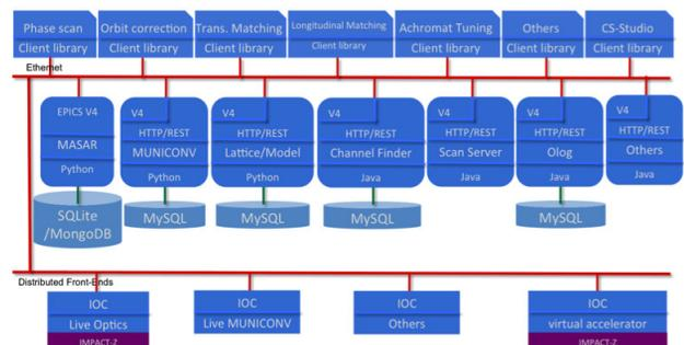
Figure 2: Planned architecture for FRIB physics application.
