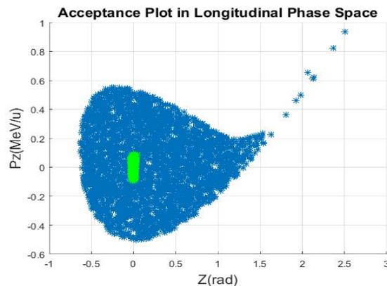
Figure 9: Longitudinal acceptance of linac segment 2.
