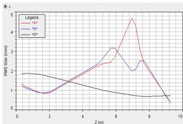
Figure 7: Beam RMS sizes after longitudinal matching
