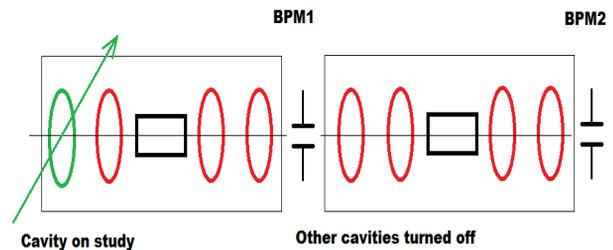
Figure 2: Schematic configuration of cavity phase scan
