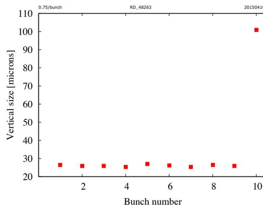
Figure 4: The vertical size of each of 10 bunches in the train, measured turn-by-turn and bunch by bunch with an xray-beam size monitor. The plotted size is a 100 turn average.
