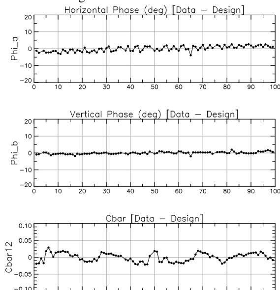
Figure 5: The turn-by-turn position of the witness bunch, measured at each of 100 beam position monitors, is used to determine betatron amplitude and phase advance.
