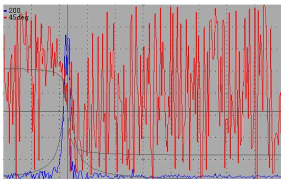
Figure 1: Frequency sweep over 10kHz. The tune tracker acquires a betatron signal by sweeping the drive frequency through a band and recording betatron amplitude and phase. Blue trace is amplitude and red trace phase response shown with fitted Lorentzian.
