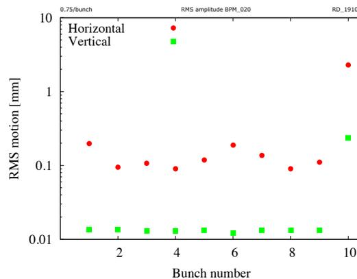
Figure 3: Standard deviation of the turn-by-turn position. The 10 bunches are spaced 14ns apart. The tune tracker is locked to the last bunch in the train, driving it at the horizontal and vertical betatron tunes.
