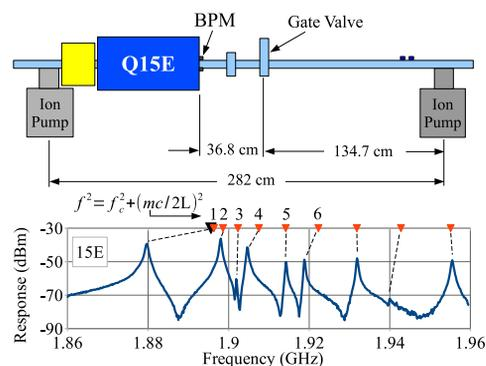
Figure 1: Sketch of the beam-pipe section at 15E along with its resonant response. Triangles show the predicted frequencies for a simple shorted waveguide. Dotted lines connect those frequencies with the measured response peaks.
