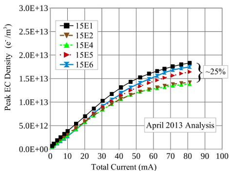
Figure 2: Data from the 15E section of CESR, showing an inconsistency of about 25% in the EC density measurements between the five modes in the same chamber. The label 15Em corresponds to mode *m*.
