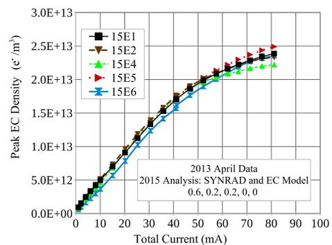
Figure 7: EC density versus beam current with corrections, using the flux, EC multiplier and  $E_0^2$  shown in Fig. 6.
