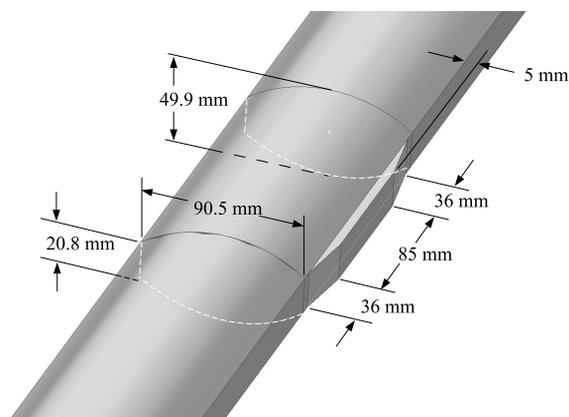
Figure 4: Model created using Inventor with some relevant dimensions. Overall dimensions (above and left) are used in the beam-pipe model. Additional dimensions that model the 5 mm recess of the gate valve body are shown at right.
