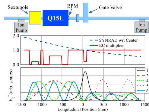
Figure 6: A sketch of the 15E section with the synchrotron radiation flux and the EC multiplier discussed in the text. The lower plots are the values of  $E_0^2$  from simulation of the relevant modes. The scale of mode 1 is altered for clarity.
