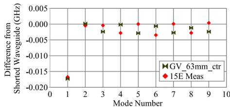
Figure 5: The simulated resonances with the gate valve 63 mm from the longitudinal center are compared with the measured peak frequencies of Fig. 1.
