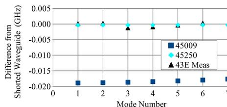
Figure 3: Comparing simulation results of two beam-pipe cross-sections and the measured response peaks at 43E. Labels are for the half-width to the beam-pipe wall in  $\mu\text{m}$ .
