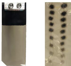
Figure 1: Primary Stripper before beam (left) and after seeing multiple beams at different currents (right) as indicated in Table 2.
