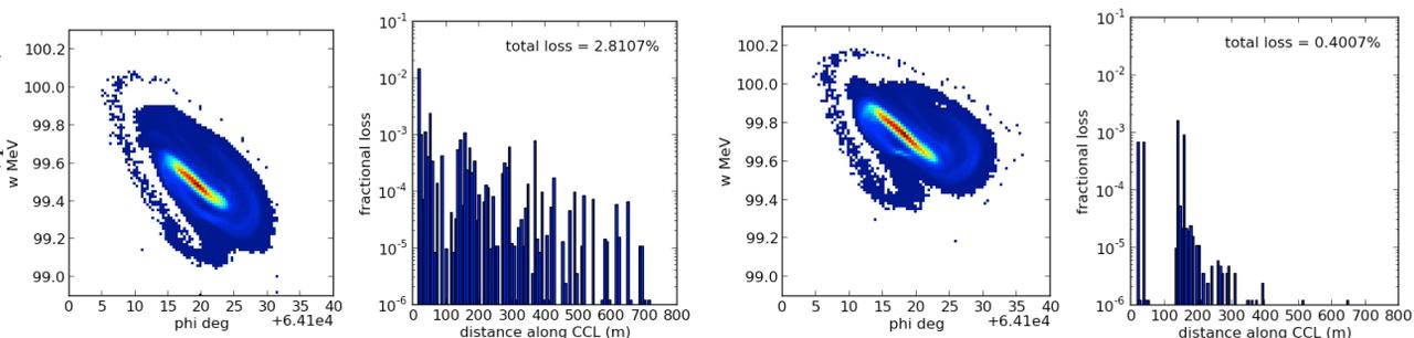
Figure 3: Simulated  $H^-$  beam distribution at the entrance to the CCL and corresponding beam loss along the CCL. Higher losses after hypothetical tuneup (left pair) and subsequent lower losses following small phase adjustment of DTL tank 3 to increase beam energy into CCL (right pair).
