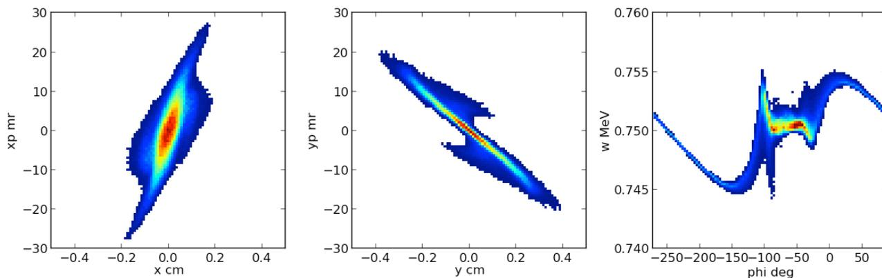
Figure 1: Simulated  $H^+$  beam transverse and longitudinal phase-space distributions at the end of the LANSCE LEBT. Color indicates intensity where red is high and blue is low.
