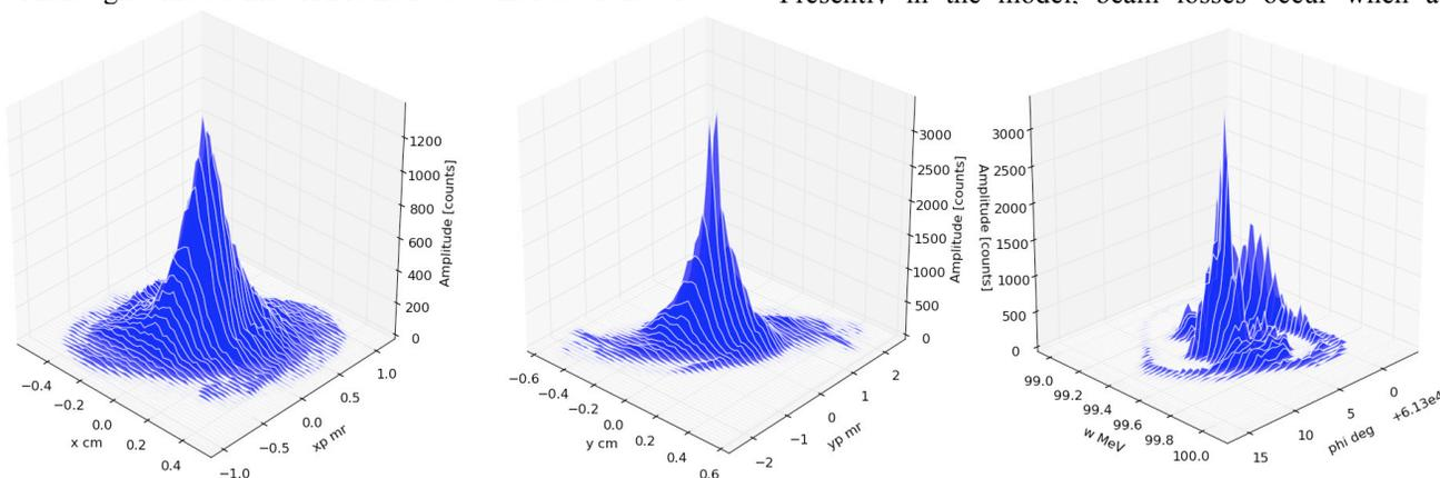
Figure 2: Simulated  $H^+$  beam transverse and longitudinal phase-space distributions at the end of the LANSCE DTL.
