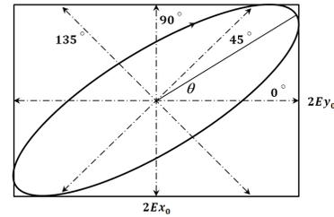
Figure 4: Beam polarization ellipse indicating polarizer orientations for Stokes' parameter measurements.  $\theta$  is the ellipse rotation angle.
