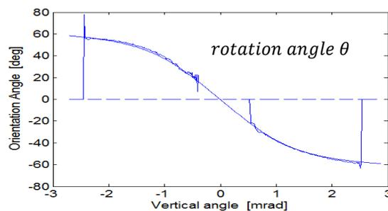
Figure 8: Polarization ellipse rotation angle as a function of vertical elevation angle.
