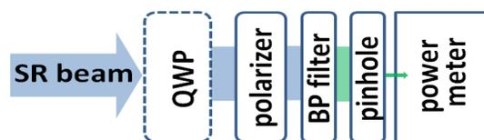
Figure 2: Stokes parameter measurement apparatus.
