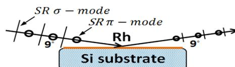
Figure 1: Visible light extraction mirror. Note E-field attenuation and relative phase shift upon reflection.
