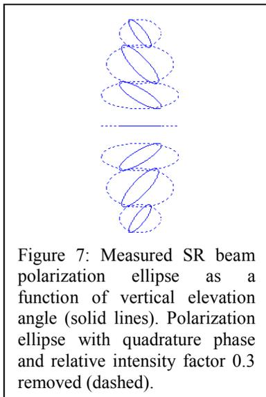
Figure 7: Measured SR beam polarization ellipse as a function of vertical elevation angle (solid lines). Polarization ellipse with quadrature phase and relative intensity factor 0.3 removed (dashed).
