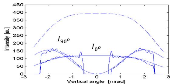
Figure 5: Horizontal (SR  $\sigma$ -mode) and vertical (SR  $\pi$ -mode) field intensities as a function of vertical elevation angle.
