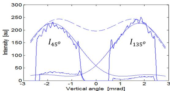
Figure 6: Field intensities measured with polarizer oriented 45° and 135° w.r.t. horizontal axis.
