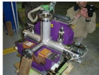
Figure 4: SPIRAL2 quadrupole used in SARAF MEBT.
