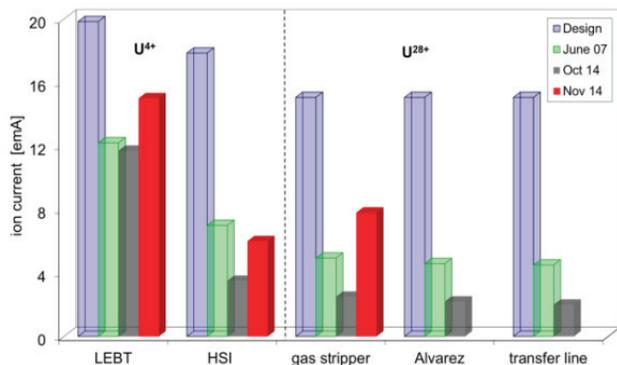
Figure 3: Achievement of a new uranium beam ( $28^+$ ) intensity record at GSI-UNILAC.
