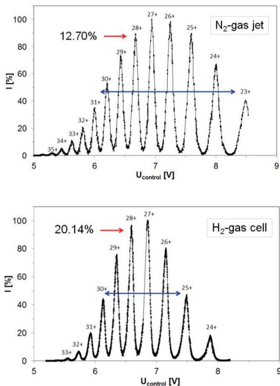
Figure 2: N<sub>2</sub>-gas jet (top) and H<sub>2</sub>-pulsed gas cell (bottom) charge spectra for max. available target density [13].
