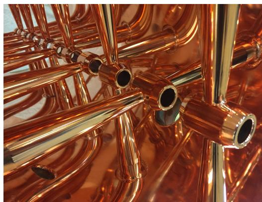
Figure 2: Picture of the copper plated inner surface of CH 3
