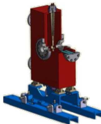
Figure 5: 3-D view of a general 2-gap buncher layout
