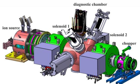
Figure 3: 3-D view of the ion source, LEBT and chopper
