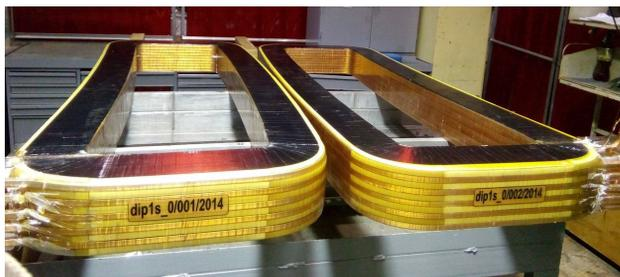
Figure 6: Set of coils for pre-series dipole magnet dip1s\_0.
