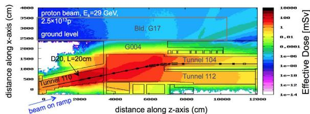
Figure 3: Effective dose for one beam pulse hitting the diffusor D20 (iron cylinder, length = 20 cm) placed along the sloped beam line section T1X2 [5].
