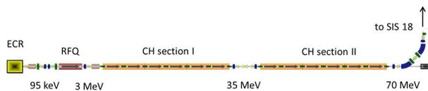
Figure 8: Schematic layout of the FAIR proton linac [3].
