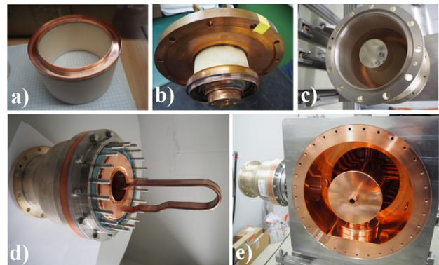
Figure 5: Coupler construction steps and final assembly.
