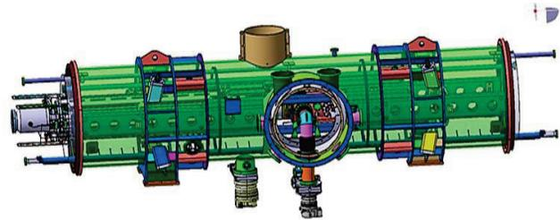
Figure 3: Manufacturing design of the quadrupole module type 2.5.
