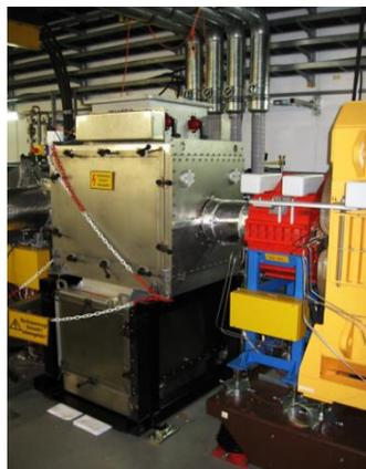
Figure 5: SIS18 MA loaded bunch compression cavity.
