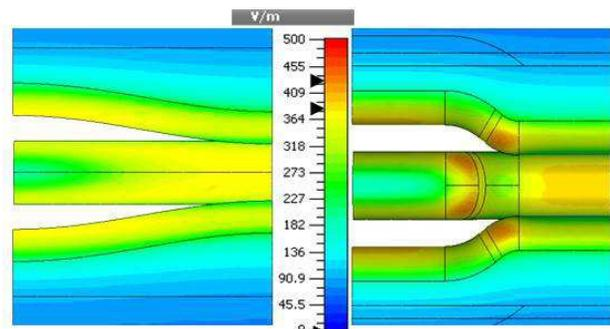
Figure 4: E-field on the CST MWS model surfaces for the sinusoidal (left) and the trapezoidal cell (right).
