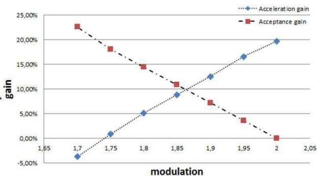
Figure 6: Acceleration and acceptance gain in dependence of the electrode cell modulation.
