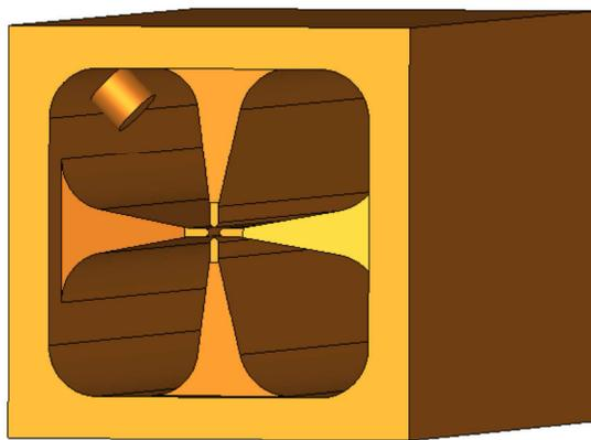
Figure 3: CST MWS model of a possible RFQ structure for the cavity design simulation.
