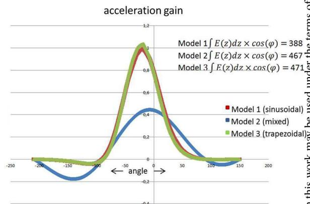
Figure 5: Effective longitudinal electric field along the Z-axis for the different models.
