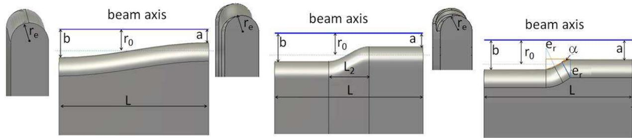
Figure 2: Layout of the three different models used for the CST MWS simulations. The main parameters are aperture (a), average distance to beam axis ( $r_0$ ), modulation ( $m=b/a$ ), cell length (L), length of the sinusoidal part ( $L_2$ ) and electrode radius ( $r_e$ ). For the trapezoidal design other parameters like edge rounding ( $e_r$ ) and an angle ( $\alpha$ ) are required.
