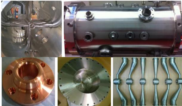
Figure 2: Manufacturing process of the cavity. Top: CH – cavity cylindrical tank. Bottom: End drift tube (left), tank end flange (middle), drift tubes structure (right).
