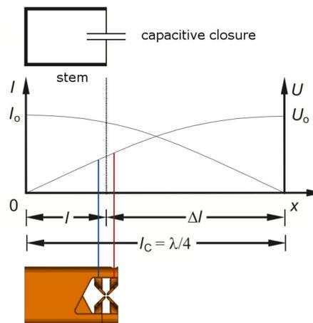
Figure 3: Description of one rf cell of an 4-rod RFQ as capacitively shortened  $\lambda/4$  resonator.
