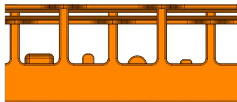
Figure 2: Different size and shapes of plunger tuners.
