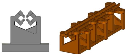
Figure 4: Approaches on dipole compensation. Adjustment of the current paths (left) and stem displacement (right).
