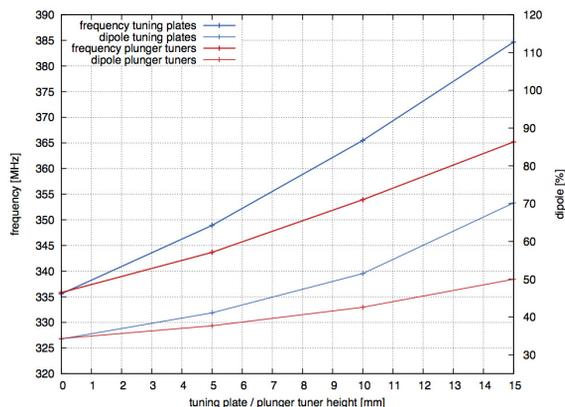
Figure 1: Comparison of common tuning plates with plunger tuner in respect to their influence on the resonant frequency and the dipole field of the RFQ.
