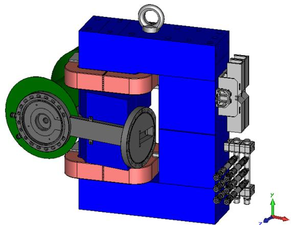
Figure 1: Model of the massless septum system for the FRANZ LEBT, consisting of a C-magnet and a shielding tube.
