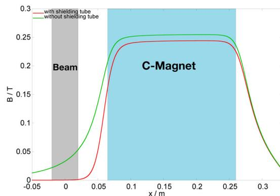
Figure 4: Magnetic field in the dipole gap with and without shielding tube.
