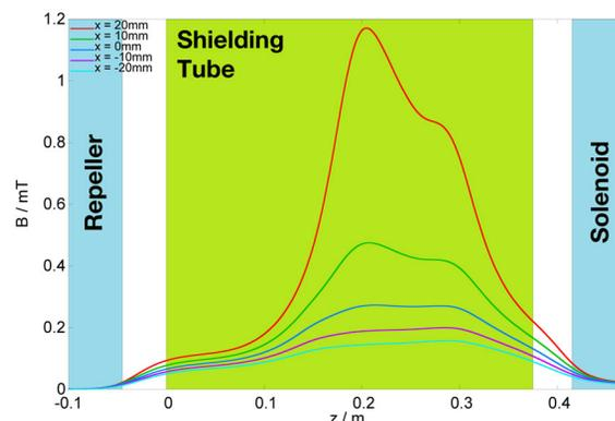
Figure 5: Magnetic field along the beam axis for different horizontal off-sets. Within 40 mm, the magnetic field increases by a factor of 10.
