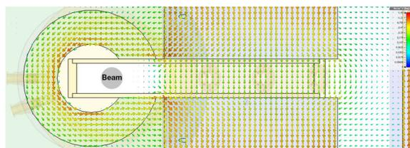
Figure 3: Transverse section of the septum system. Magnetic field lines visualize the magnetic flux.
