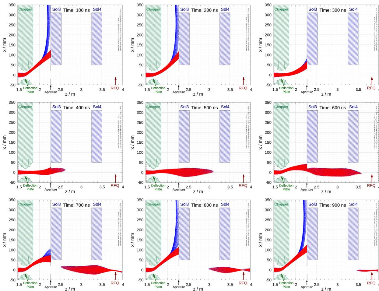
Figure 6: Sweep of the 120 keV, 50 mA proton beam during the HV pulse of the chopper's electric deflector, with (blue) and without (red) septum system [3].
