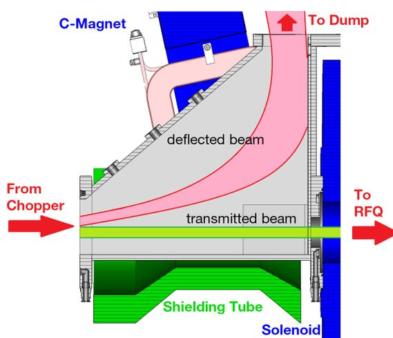
Figure 2: Horizontal cross section of the septum system including the vacuum chamber. The C-magnet will extract the deflected beam out of the beamline and guide it into a beam dump. The shielding tube will reduce the magnet's fringing field on the beam axis of the transmitted beam.
