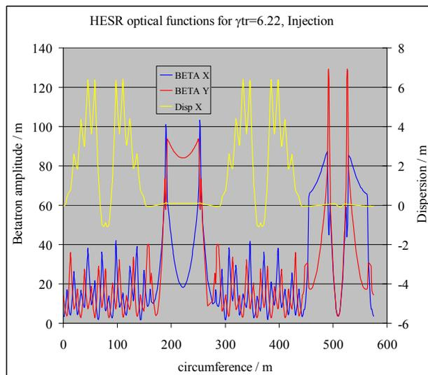
Figure 2: Optical functions for the HESR magnet lattice with dispersion suppression for transition energy of  $\gamma_{tr}=6.22$ . Shown are the horizontal betatron amplitude  $\beta_x$  (blue), the vertical betatron amplitude  $\beta_y$  (red), and the horizontal dispersion  $D_x$  (yellow) along the ring.
