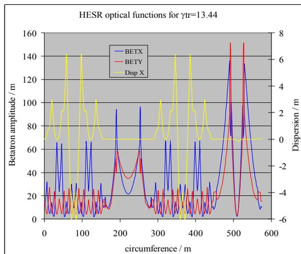
Figure 3: Optical functions for the HESR magnet lattice with dispersion suppression for transition energy of  $\gamma_{tr}=13.4$ . Shown are the horizontal betatron amplitude  $\beta_x$  (blue), the vertical betatron amplitude  $\beta_y$  (red), and the horizontal dispersion  $D_x$  (yellow) along the ring.
