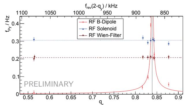
Figure 5: Results of the resonance scans at the nominal tune of COSY at  $Q_y = 3.56$  and for a set of vertical betatron tunes with sideband frequencies around the spin resonance, depicted by the vertical line at 871 428.00 Hz.
