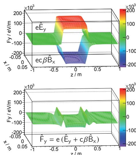
Figure 2: Simulation of the *Lorentz-Force* on a particle entering the RF ExB-Dipole on axis across a horizontal cut through the center of the beam pipe. The results have been normalized to a coil current amplitude of  $\hat{I} = 1$  A.
